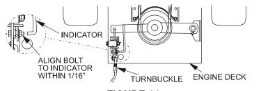
FIGURE 14 PTO ENGAGEMENT LINKAGE
